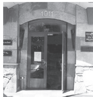
FIG. 12 - CREATE EASILY IDENTIFIABLE BUILDING ENTRANCES. RECESS BUILDING ENTRIES TO ACCOMMODATE OUTWARD DOOR SWINGS.
