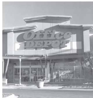
FIG. 11 - TERMINATE THE TOP OF FLAT ROOF BUILDINGS WITH A DISCERNABLE ROOF CAP. USE AMPLE CORNICE ELEMENTS AND PARAPET WALLS TO TOP THE BUILDING.
