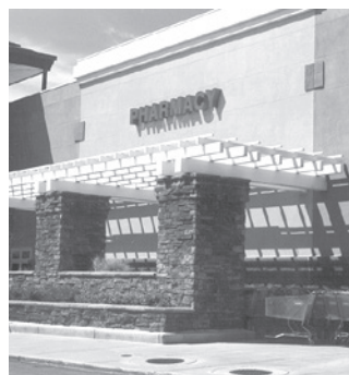
FIG. 8 - USE TRELLIS ELEMENTS TO SOFTEN LARGE FORMAT ARCHITECTURE. NOTICE HOW THE SUBSTANTIAL STONE PIER AND DIMENSIONAL TIMBER TRELLIS STRUCTURE ADDS FAÇADE VARIETY AND VISUAL INTEREST. NOTICE ALSO THAT CART STORAGE IS SCREENED FROM PUBLIC VIEW.
