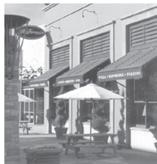
FIG. 10 - DESIGN STOREFRONT AWNINGS TO CONFORM TO INDIVIDUAL STRUCTURAL BAYS. CONTINUOUS AWNINGS SHALL BE AVOIDED.
